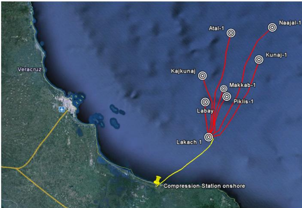
Figure 9.5: Location of prospects and hypothetical paths of pipelines if Lakach would have been developed as a processing Hub for future field developments in this gas province.
