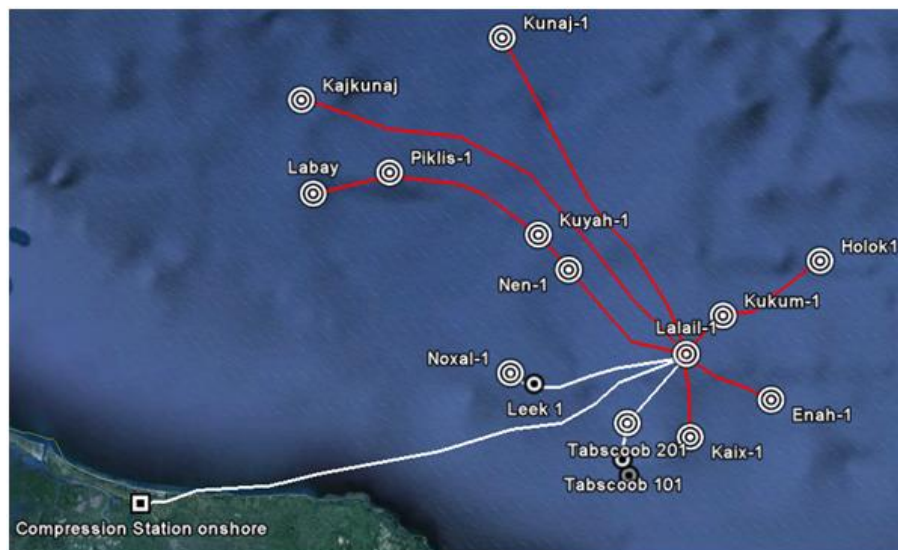
Figure 9.7: Hypothetical development for a Floating structure in Lalail also as a Hub for the future field developments of this gas province.
