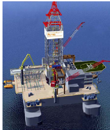
Figure 6.b The semisubmersible rig "Petrorig 1" [Petromena, 2007]
